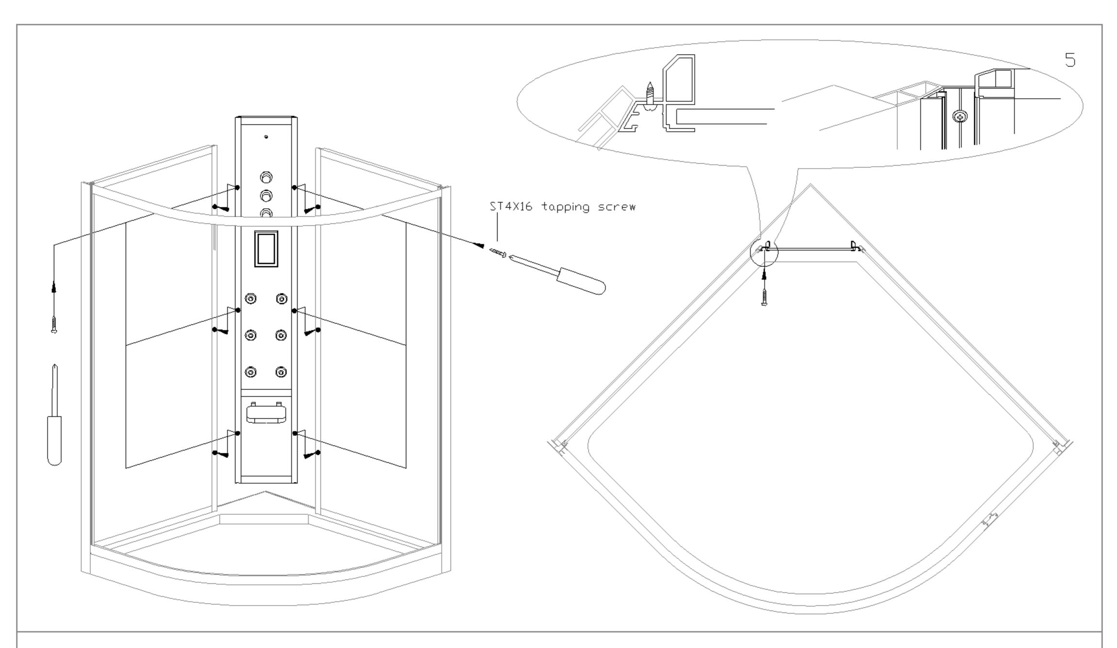
Install the middle back panelGet the middle back panel connected to the glass back wall with tapping screws.
