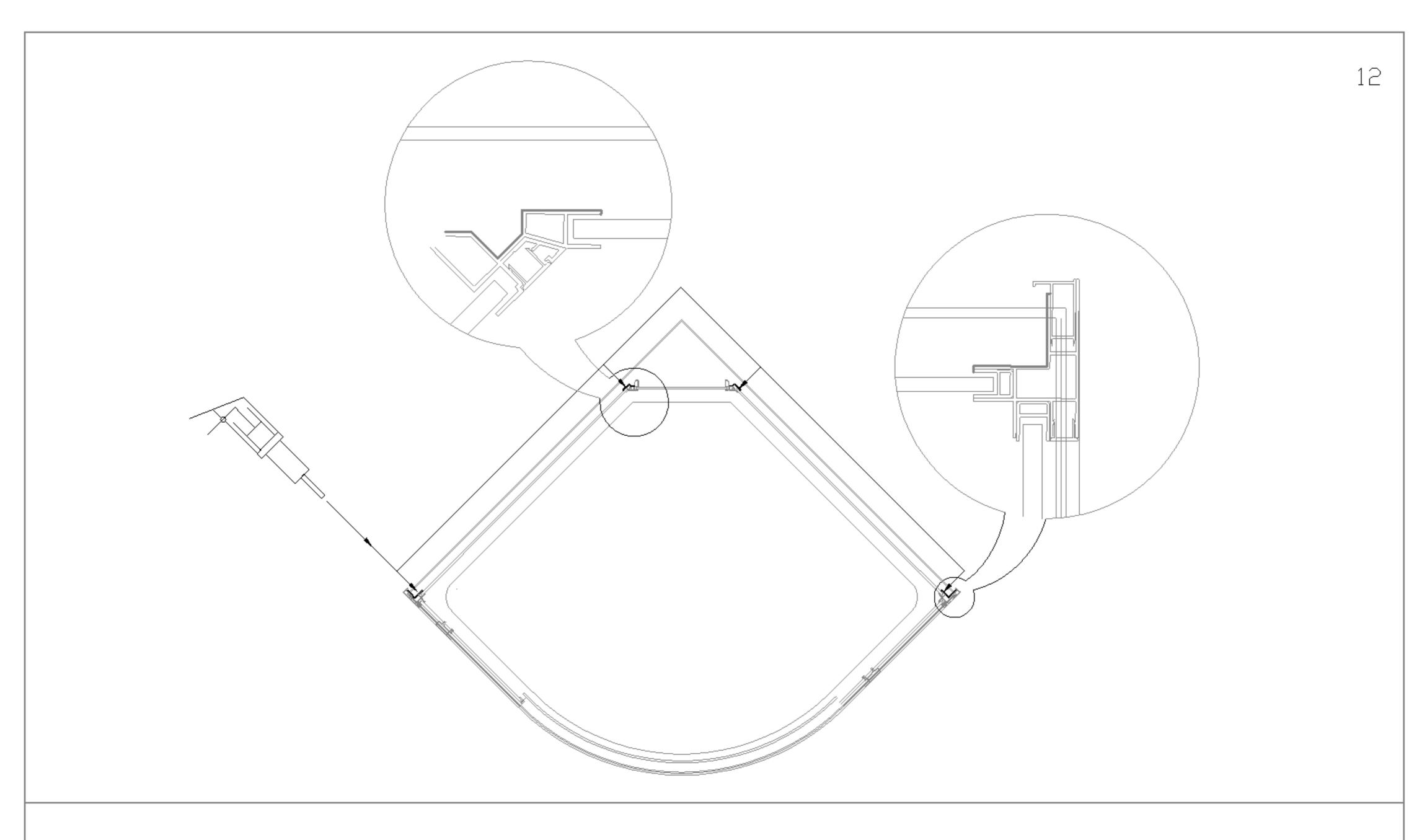
12. Apply silicone. No using within 24 hours.
