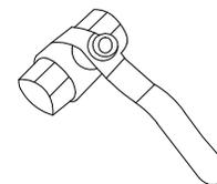
RECOMMENDED - SHUT OFF VALVES FOR HOT AND COLD
